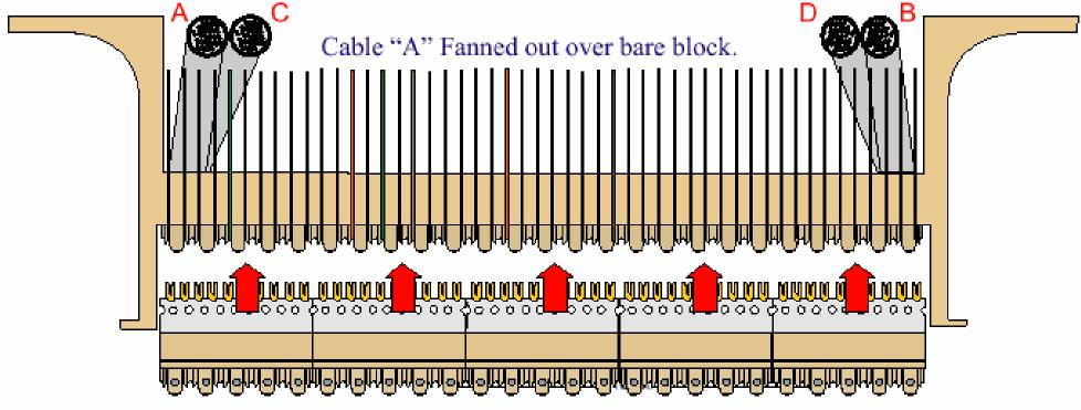
(5) 110C5's are punched over conductors to terminate cable pairs with a 5-Pair punch down tool.
